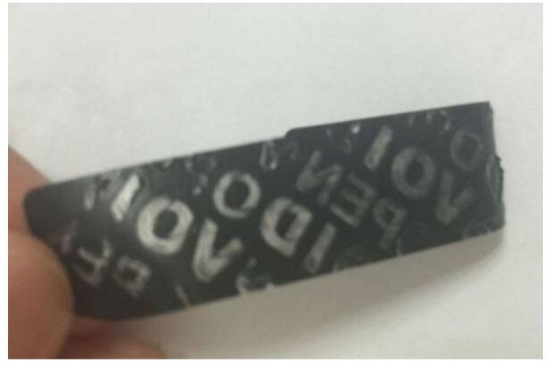
The Void label has a hidden message revealed in the plastic film when the label is removed. Its featur include:
